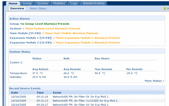
Figure 6 APC Network Air FM web interface
